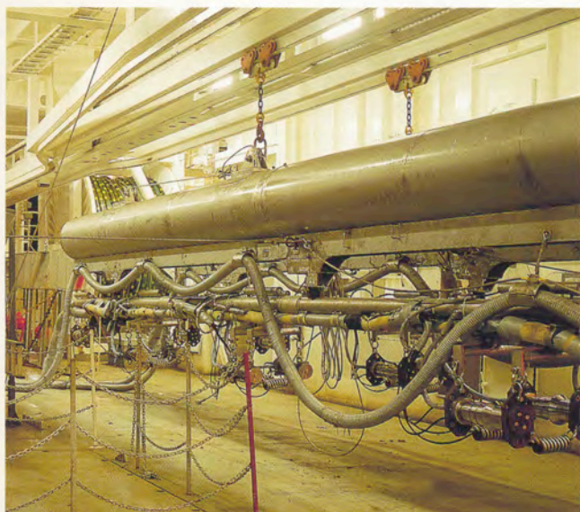
Sleeve airgun on board M/V CGG Mistral.
