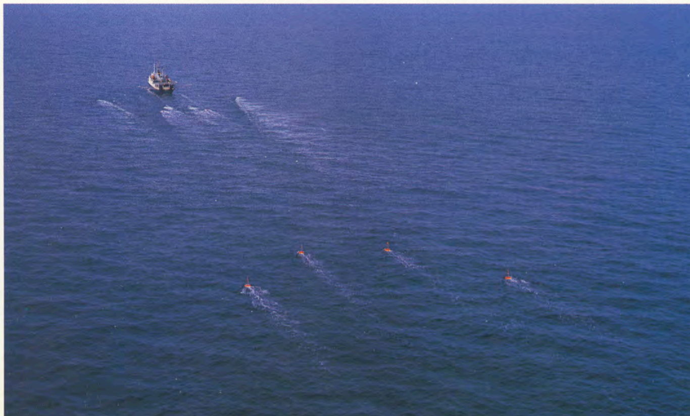
The M/V Stormy during operations in the North Sea with four short streamers.
