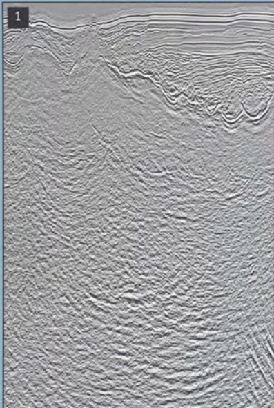
▲ Figure 1: Time migration image illustrating the difficulties of accurate sub-salt interpretation.
