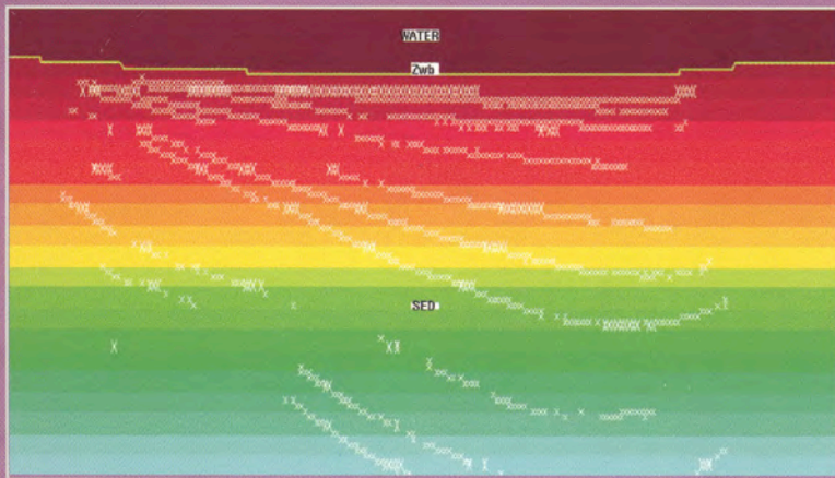
◀ Initial inversion velocity model showing RMO analysis locations (white crosses)
