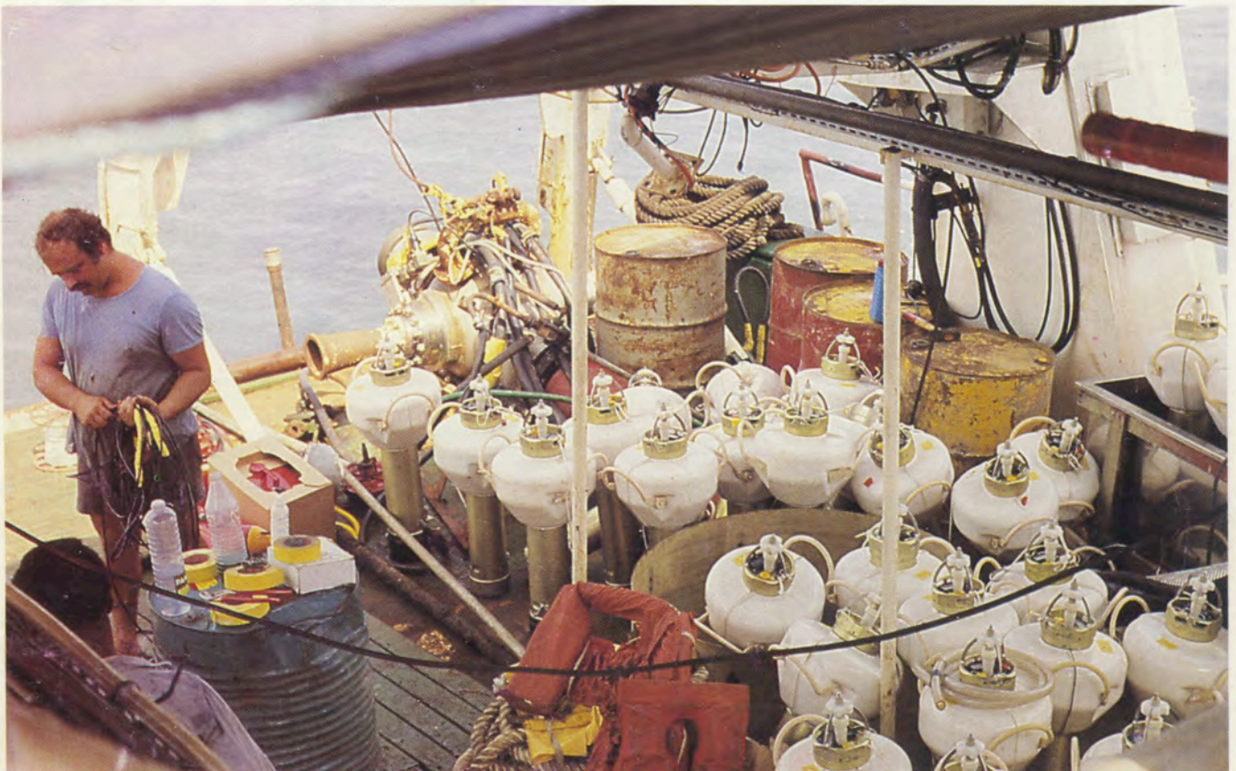
Myriaseis radiotelemetry station units ready to be launched into the water during a land/sea transition zone survey.
